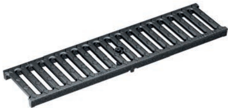
Slotted grating SW 10, ductile-iron, cataphoretic dip coating Load class: C250 , Lenght: 50 cm, SW 10 mm
