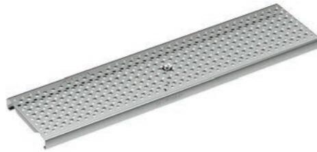
Perforated grating, galvanised, stainless steel Load classes: A15, C250 , Lenght: 50 cm, 100 cm, Ø 6 mm
