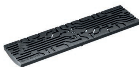
Design grating, WIRE Design, ductile-iron, cataphoretic dip coating Load class: D400* , Lenght: 50 cm, SW 5 mm
