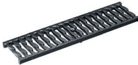
Slotted grating, OvalGrip Design, ductile-iron, cataphoretic dip coating Load classes: C250, E600* , Lenght: 50 cm, SW 10 mm
