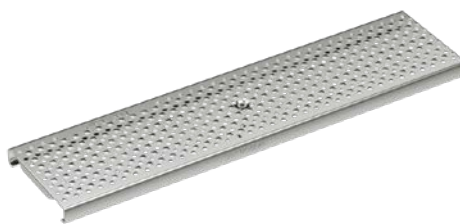
Perforated grating, galvanised, stainless steel Load classes: A15, C250 , Lenght: 50 cm, 100 cm, Ø 6 mm
