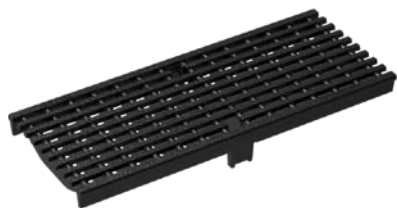
Longitudinal-bar grating, ductile-iron GJS, cataphoretic dip coating Load classes: E600* Lenght: 50 cm, MW 25 x 11 mm
