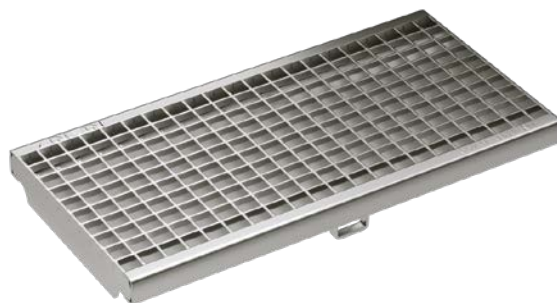
Mesh grating, galvanised, stainless steel Load classes: D400* Length: 50 cm, 100 cm, MW 20 x 20 mm
