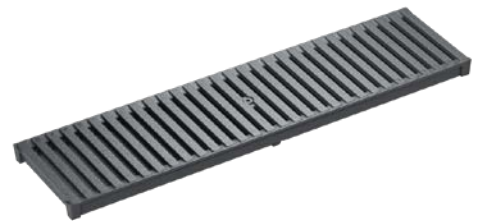
Slotted grating, HEELGUARD, ductile-iron, coated in black Load class: D400* , Lenght: 50 cm, SW 6 mm
