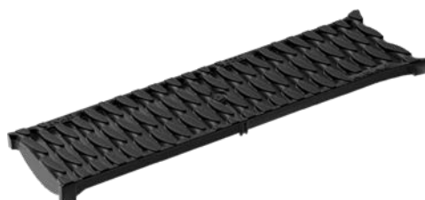
Slotted grating, OvalGrip Design, polyamide, black Load class: C250 , Lenght: 50 cm, SW 8 mm
