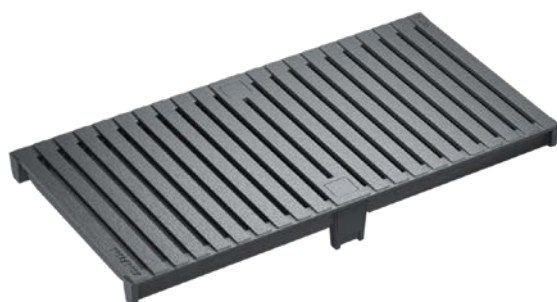
Slotted grating, HEELGUARD, ductile-iron GJS, black coating or cataphoretic dip coating, Load classes: D400* , Length: 50 cm, SW 6 mm
