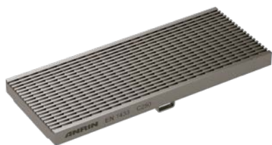
Longitudinal profile grating, stainless Load class: C250 Lenght: 50 cm, 100 cm, SW 5 mm
