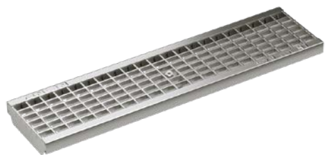
Mesh grating, galvanised, stainless steel Load classes: B125, C250, D400 , Lenght: 50 cm, 100 cm MW 30 x 14 mm / 30 x 10 mm / 20 x 14 mm
