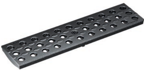
Design grating, CIRCLE, GJS ductile-iron, cataphoretic dip coating Load class: D400 , Lenght: 50 cm, Ø 19,5 mm
