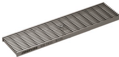
Longitudinal profile grating, stainless steel Load classes: B125, D400 , Lenght: 50 cm, 100 cm, SW 5 mm
