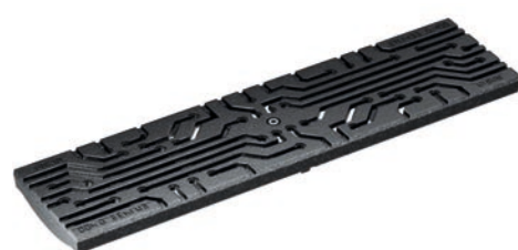
Design grating, WIRE Design, ductile-iron, cataphoretic dip coating Load class: D400* , Lenght: 50 cm, SW 5 mm
