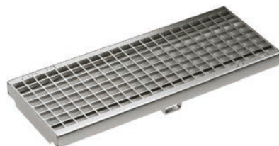
Mesh grating, galvanised, stainless steel Load classes: C250, D400* Lenght: 50 cm, 100 cm, 20 x 20 mm
