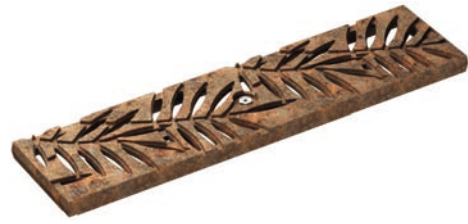
Design grating, LEAF, ductile-iron, uncoated Load class: C250 , Lenght: 50 cm, SW 5 - 9 mm
