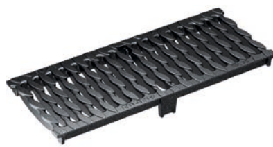
Slotted grating with OvalGrip Design, ductile-iron GJS, cataphoretic dip coating Load classes: D400*, E600* Lenght: 50 cm, SW 12 mm
