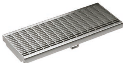
Mesh grating, galvanised, stainless Load classes: C250 Lenght: 50 cm, 100 cm, MW 30 x 10 mm
