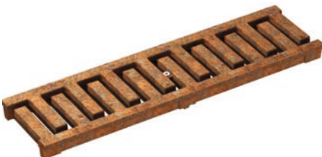
Slotted grating, MASSIV 32, ductile-iron, uncoated Load class: E600* , Lenght: 50 cm, SW 11 mm Only suitable for KE-100.
