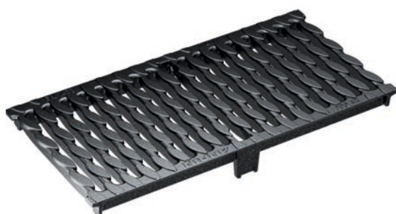
Slotted grating with OvalGrip Design, ductile-iron GJS, cataphoretic dip coating Load classes: D400* , E600* , Length: 50 cm, SW 12 mm
