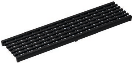
Longitudinal-bar grating, ductile-iron, cataphoretic dip coating Load class: D400* , Lenght: 50 cm, MW 25 x 10 mm
