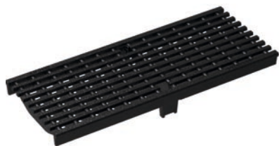
Longitudinal-bar grating, ductile-iron GJS, cataphoretic dip coating Load classes: D400*, E600* Lenght: 50 cm, MW 25 x 11 mm
