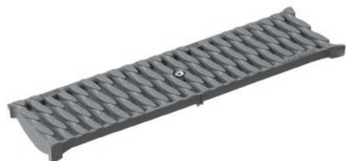
Slotted grating, OvalGrip Design, polyamide, gray Load class: B125 and C250 , Lenght: 50 cm, SW 8 mm
