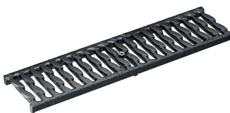
Slotted grating, OvalGrip Design, ductile-iron, cataphoretic dip coating Load classes: C250, E600* , Lenght: 50 cm, SW 10 mm Load class: F900 only for channel KF-100
