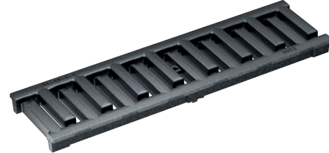
Slotted grating, MASSIV 32, ductile-iron, cataphoretic dip coating Load class: E600* , Lenght: 50 cm, SW 11 mm Only suitable for KE-100.
