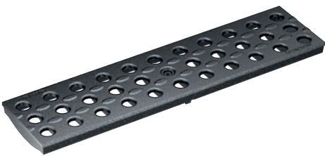
Design grating, CIRCLE, GJS ductile-iron, cataphoretic dip coating Load class: D400 , Lenght: 50 cm, Ø 19,5 mm
