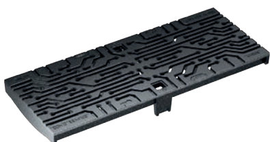
Design grating, WIRE, ductile-iron GJS, cataphoretic dip coating Load class: D400* Lenght: 50 cm, SW 5 mm
