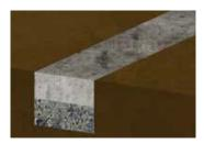
3. Fill concrete, 3 parts sand + 1 part water + 1 part cement, into the base of the trench.
