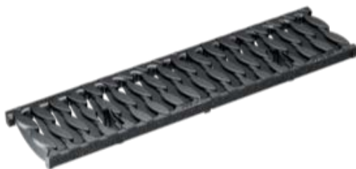
Slotted grating, OvalGrip Design, ductile-iron, cataphoretic dip coating Load classes: F900 Length: 50 cm, SW 10 mm with RapidLock fastening
