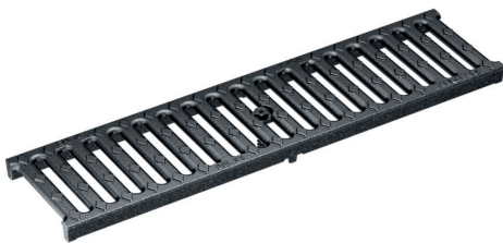
Slotted grating SW 10, ductile-iron, cataphoretic dip coating Load class: C250 , Length: 50 cm, SW 10 mm
