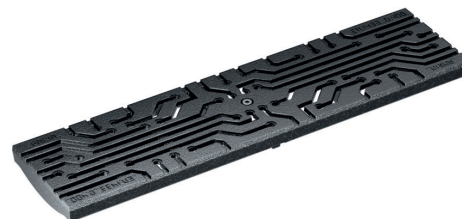
Design grating, WIRE Design, ductile-iron, cataphoretic dip coating Load class: D400* , Length: 50 cm, SW 5 mm
