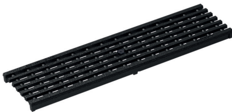
Longitudinal-bar grating, ductile-iron, cataphoretic dip coating Load class: D400* , Length: 50 cm, MW 25 x 10 mm
