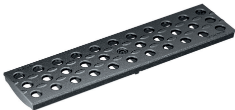
Design grating, CIRCLE, GJS ductile-iron, cataphoretic dip coating Load class: D400 , Length: 50 cm, Ø 19,5 mm
