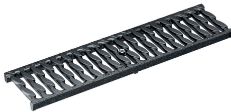
Slotted grating, OvalGrip Design, ductile-iron, cataphoretic dip coating Load classes: C250, E600* , Length: 50 cm, SW 10 mm
