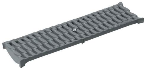
Slotted grating, OvalGrip Design, polyamide, gray Load class: B125 , Length: 50 cm, SW 8 mm
