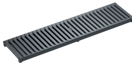
Slotted grating, HEELGUARD, ductile-iron, coated in black Load class: D400* , Length: 50 cm, SW 6 mm
