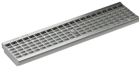
Mesh grating, galvanised, stainless steel Load classes: B125, C250, D400 , Length: 50 cm, 100 cm MW 30 x 14 mm / 30 x 10 mm / 20 x 14 mm
